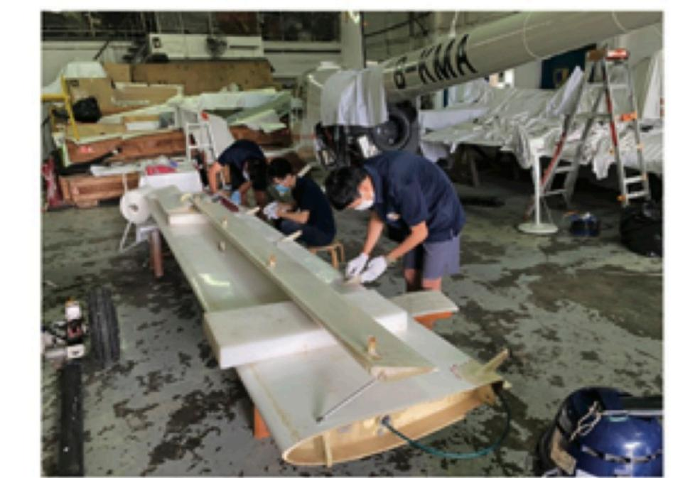
Image 16. Drilling and blind riveting
