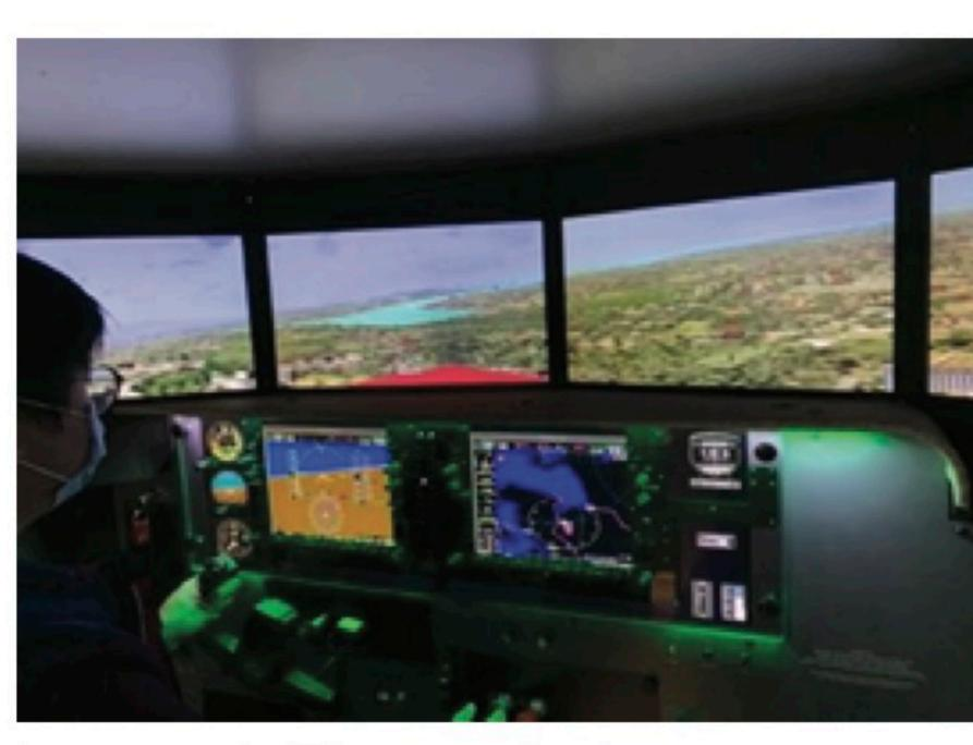
The AATD can provide a realistic training environment like 3-axis motion and wrap-around visual effect. It can simulate pitch, roll and yaw real-time movements of a plane (Image 5).
