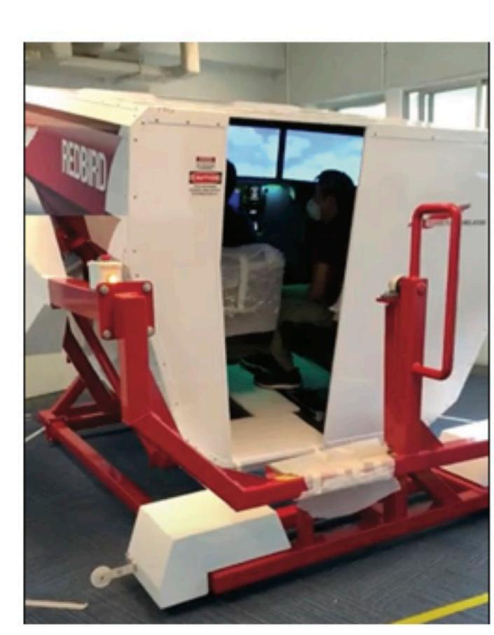
Image 5. Pitching motion of the Redbird FMX
