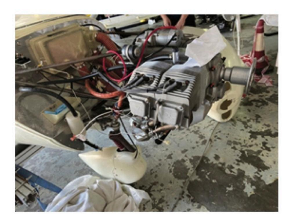
Image 19. Assembling the engine
